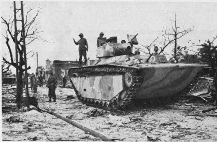
LVT(A)4 at Saipan has stubby, 75-mm. howitzer instead of 37-mm. gun found on the LVT(A)1. Redesigned turret has rear overhang.
